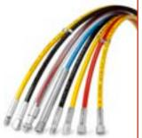
70 MPa (DN 6) - Inner tube of polyamide (PA), 2 spiral layers of high tensile steel wire, 2 open spiral synthetic fibre, outer sheath of polyurethane (PUR)
