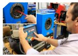
HOSE CRIMPING Each High-Pressure Center features a hose crimping facility that assembles hose kits to customer orders.
