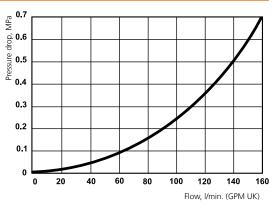
Flow measured with coupling Series 665
