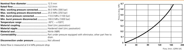
Rated flow is measured at 0.4 MPa pressure drop.
