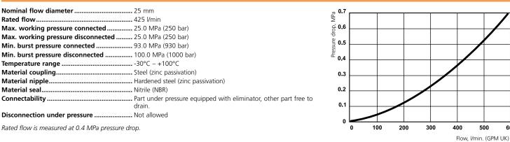
Connection Part No. Length Diameter Hexagon Seal COUPLINGS 105251209 92 NBR Female thread G 1" 62 48 105251219 G 1" 92 62 48 **FPM** COUPLINGS Female thread 105250209 G 1″ 92 62 48 NBR WITHOUT VALVE COUPLINGS NBR Female thread 105251239 G 1" 92 62 48 WITH PRESSURE ELIMINATOR NIPPLES Female thread 105256209 G 1″ 56.5 48 45 NBR 105256219 56.5 48 45 FPM G 1" NIPPLES WITHOUT G 1″ Female thread 48 45 105255209 56.5 VALVE **NIPPLES WITH** Female thread 105256239 G 1″ 56.5 48 45 NBR
