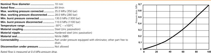
Rated flow is measured at 0.4 MPa pressure drop.
