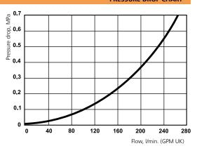
Rated flow is measured at 0.1 MPa pressure drop.
