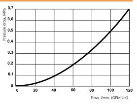
Flow measured with coupling Series 565
