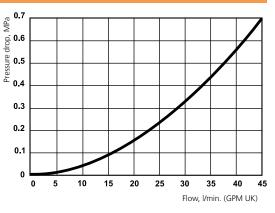
Flow measured with coupling Series 365
