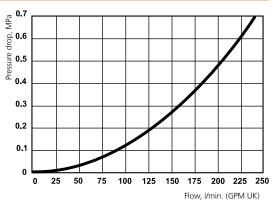
Flow measured with coupling Series 765
