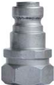
Wear to nipple caused by Locking Balls on the coupling
