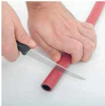
Inorder to keep the hose in the correct angle cut it with a sharp knife or hose cutter (SAS26).
