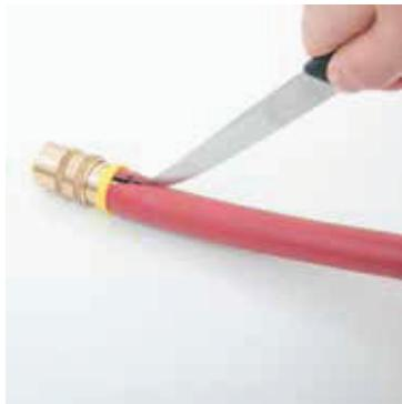
Slightly cut the hose with a knife on the longitudinal axis. Pay attention not to damage the nipple.
