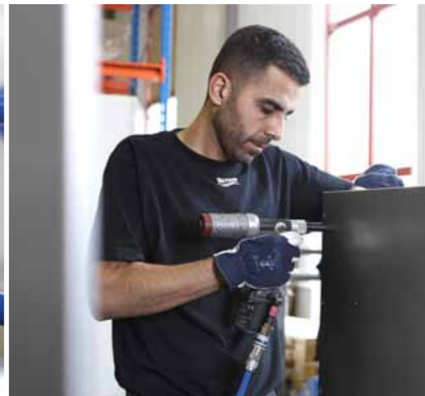
eSafe vents the down streaming pressure before disconnection reducing noise level and the risk of operator injury during tool change.
